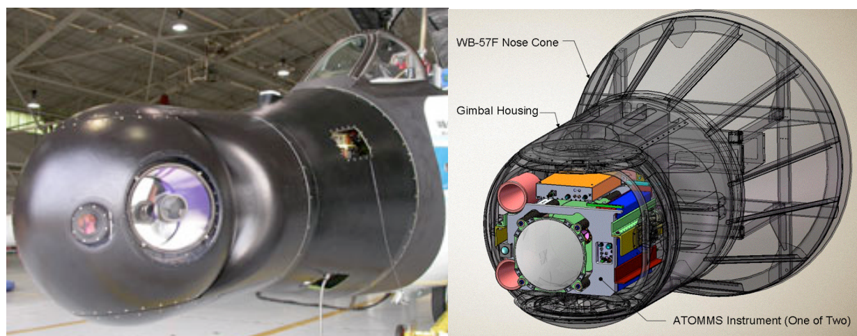
Fig. 6. Left hand panel: WB-57F aircraft with gymbal nose cone. Right hand panel: ATOMMS instrument mounted in the nose cone gymbal.
